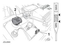
Remove the dipstick (1) and wipe clean with a non-fluffy cloth. Replace fully, then withdraw the dipstick. If the oil level is above the minimum mark on the dipstick then no additional oil is required.
