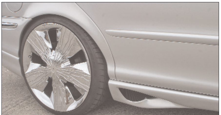
Massive US 20" alloys are unusual in their design, as is the individual air scoop treatment to the rear of the sills. Apparently Mike Hickmaw of Spray Station hand-made these out of drain-pipes!
