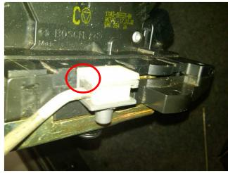
White Plastic Connector Open, Releasing Metal Linkage
