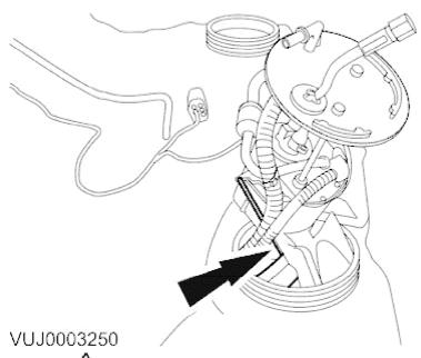
Make sure the float or arm are not damaged while removing the fuel pump module.
