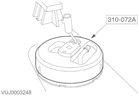
11. Using the special tool, remove the locking ring.
