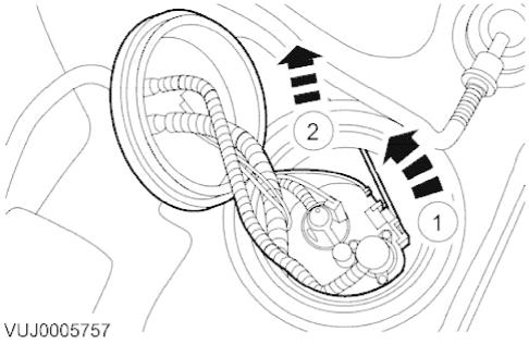
Make sure the float or arm are not damaged while removing the fuel pump module.
