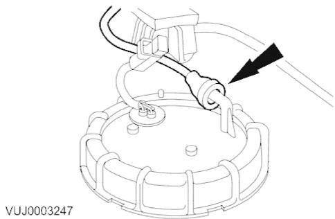
10. Disconnect the fuel supply pipe.
