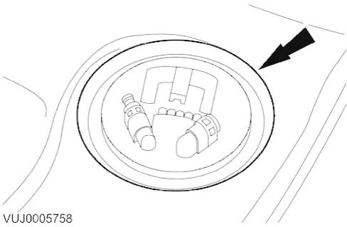
6. Detach the top of the fuel pump module.
