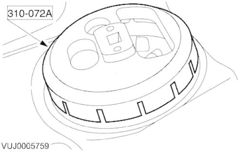
5. Using the special tool, remove the locking ring.
