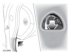
In the event of an accident, an inertia switch may trip, isolating fuel pump operation. Once the switch has tripped it must be reset before attempting to restart the engine.
