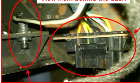
OBD II Diagnostic Plug (Under Dash on Driver's Side)
