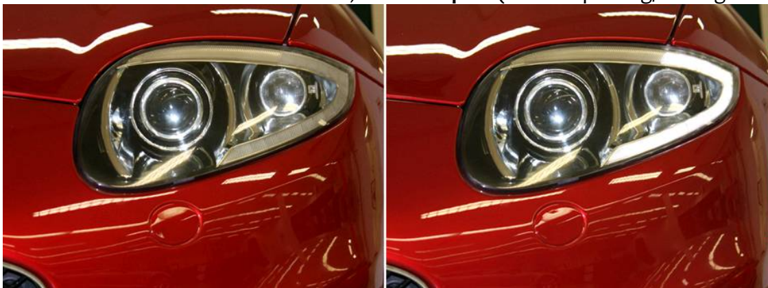
The new 2012MY headlamp shown with (right) and without (left) the LEDs illuminated
