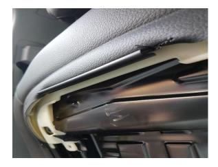
3. Open the centre console and using the panel tool gentle lift the audio connection panel out, being careful not to damage the clips circled red. Once this is removed carefully slide the power cable through the hole and down between the side panel and the seat. I used a small file just to make a notch in the side of the hole so when replacing the panel, it would not pinch the cable.
