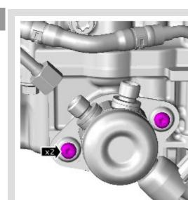
Loosen the Torx screws half a turn each.
