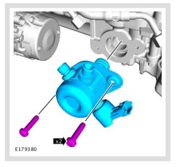
Install the high-pressure fuel pump. *Torque:* **12 Nm**
