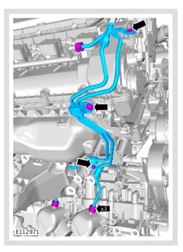
Install the high-pressure fuel supply lines, tighten the bolts and unions finger tight at stage.
