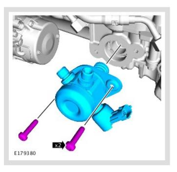
Loosen the Torx screws a turn each at a time.
