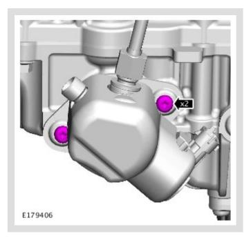
Tighten the Torx screws. Torque: **12 Nm**
