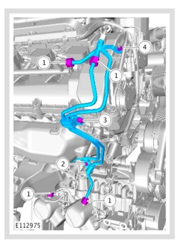
Unions (1) **21 Nm** M6 (2) **11 Nm** M8 (3) **25 Nm** M5 nut (4) **6 Nm**
