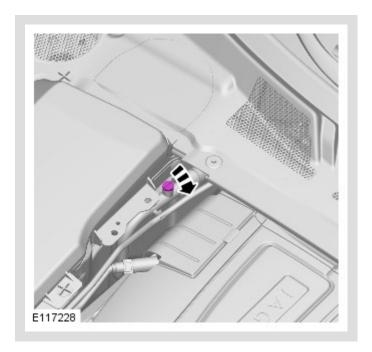
Fill the cooling system, keeping coolant to the upper level mark of the expansion tank until a steady stream of coolant is seen running from the coolant hose bleed point.
