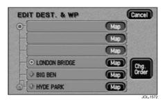
After touching **List**, the list showing the stored way points and destination (if entered) is displayed. The first way point to be visited is at the bottom of the list and the destination at the top.
