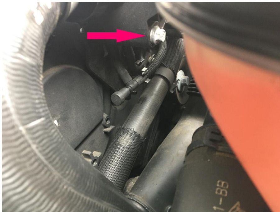
Location of bolt holding the air box on
