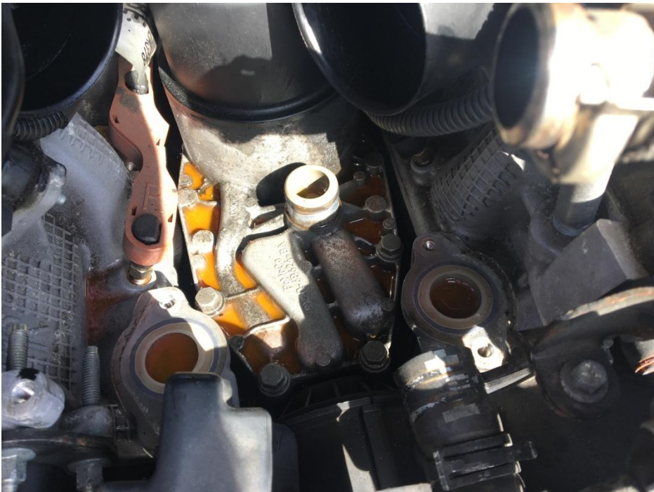
Water outlet removed
