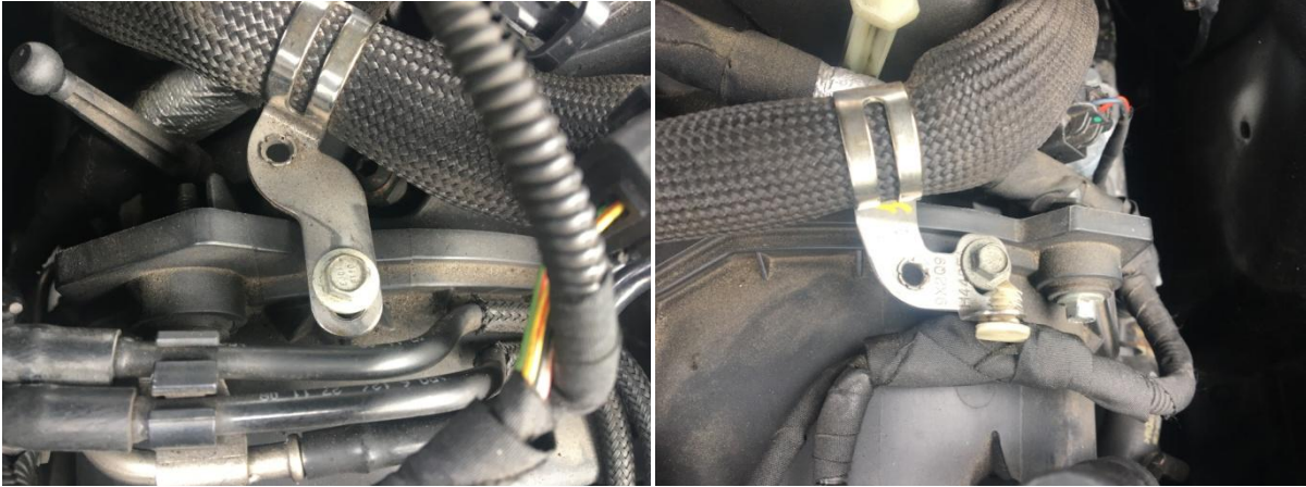
EGR valve outlet tube securing bolts
