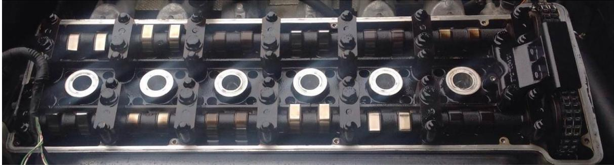
Using a 33mm spanner rotate engine to top dead centre, you will see a little "blob" in the window on the cam sensor, rotate till it is in the middle of the window. DO NOT ROTATE AGAIN
