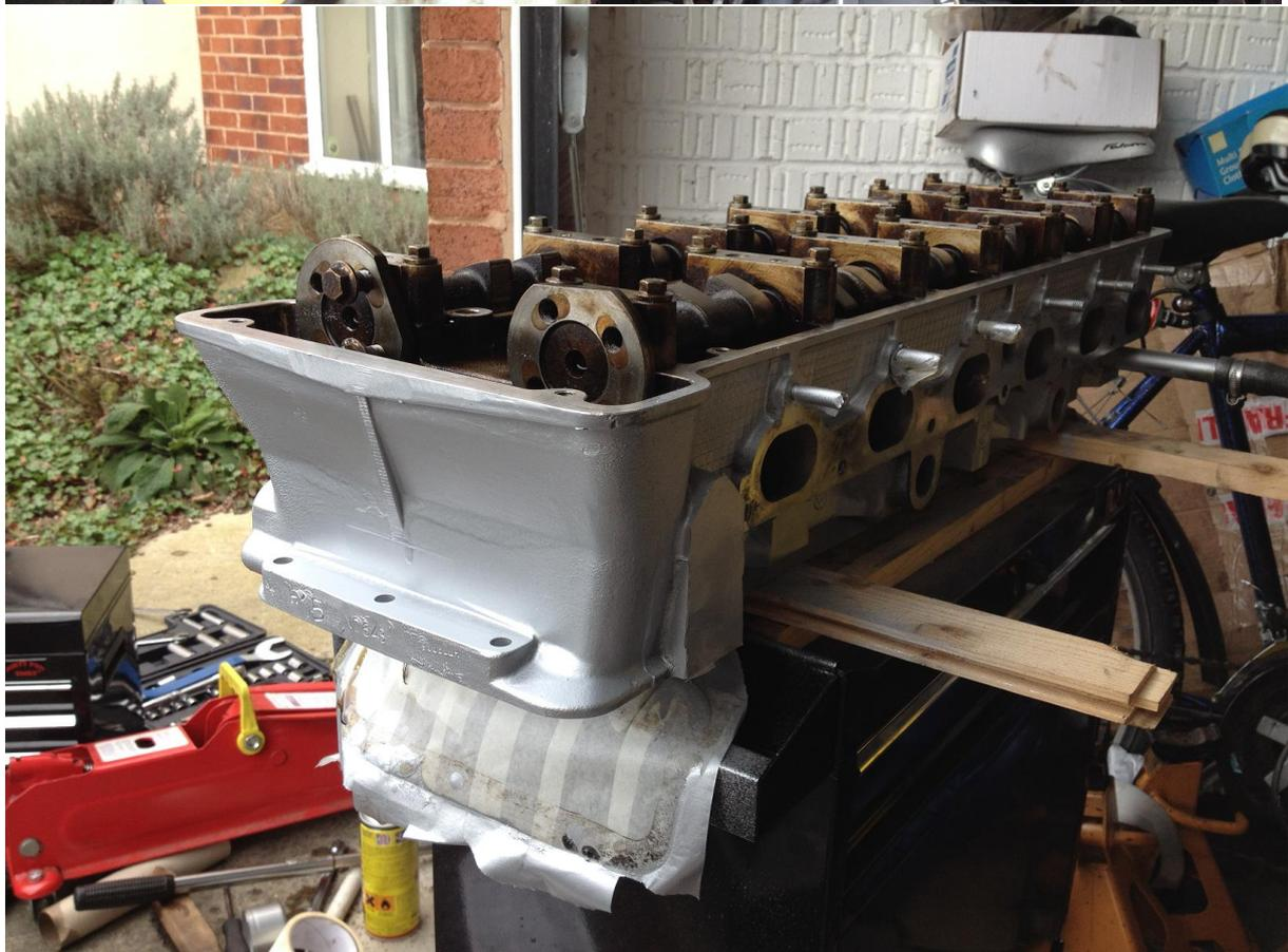
That pipe on the right of the head needs a bit of a wiggle to get out! Remember to put head on slats and NOT put flat on a surface as valves are sticking down.
