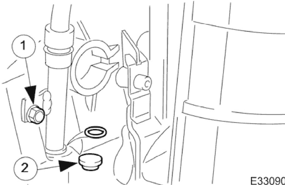
37. Remove the transmission dipstick tube.
