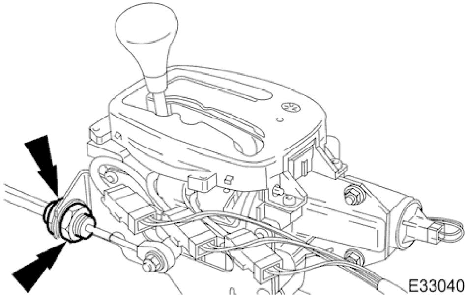
6. Slacken the selector cable locking nuts away from the abutment.
