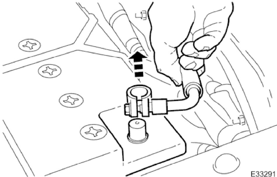
1. Disconnect battery ground cable.
