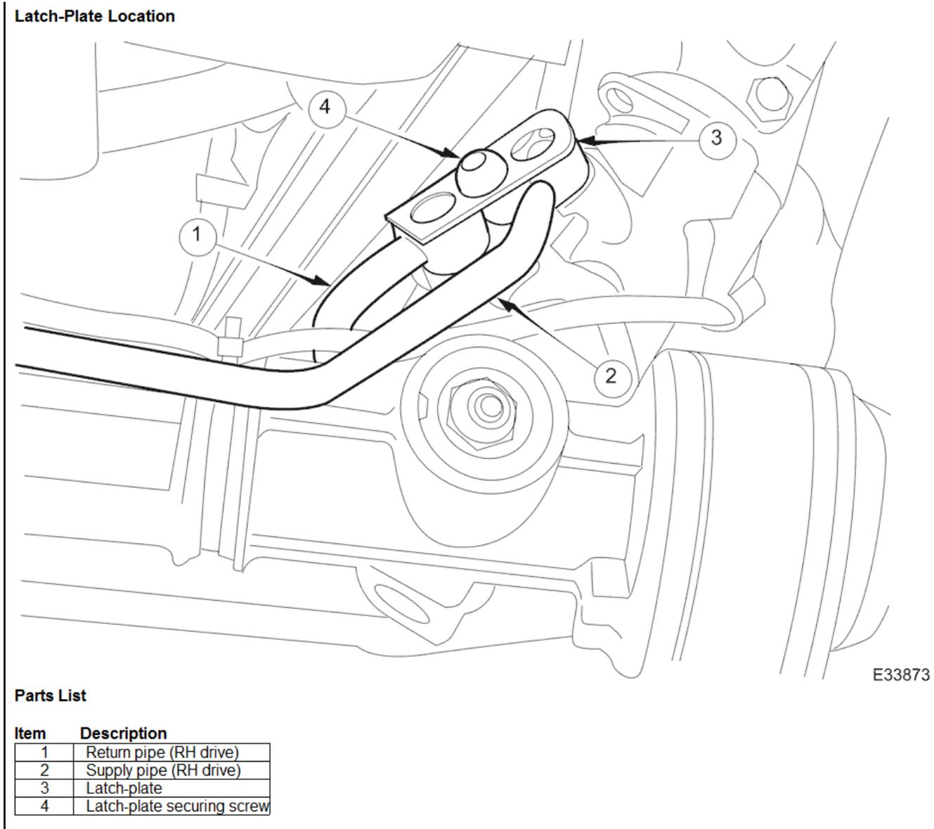
The supply and return pipes are secured to the hydraulic control valve housing by a latch-plate having a single fixing screw. The latch-plate is captive to the supply pipe. Each pipe has an O-ring which is a serviceable item.
