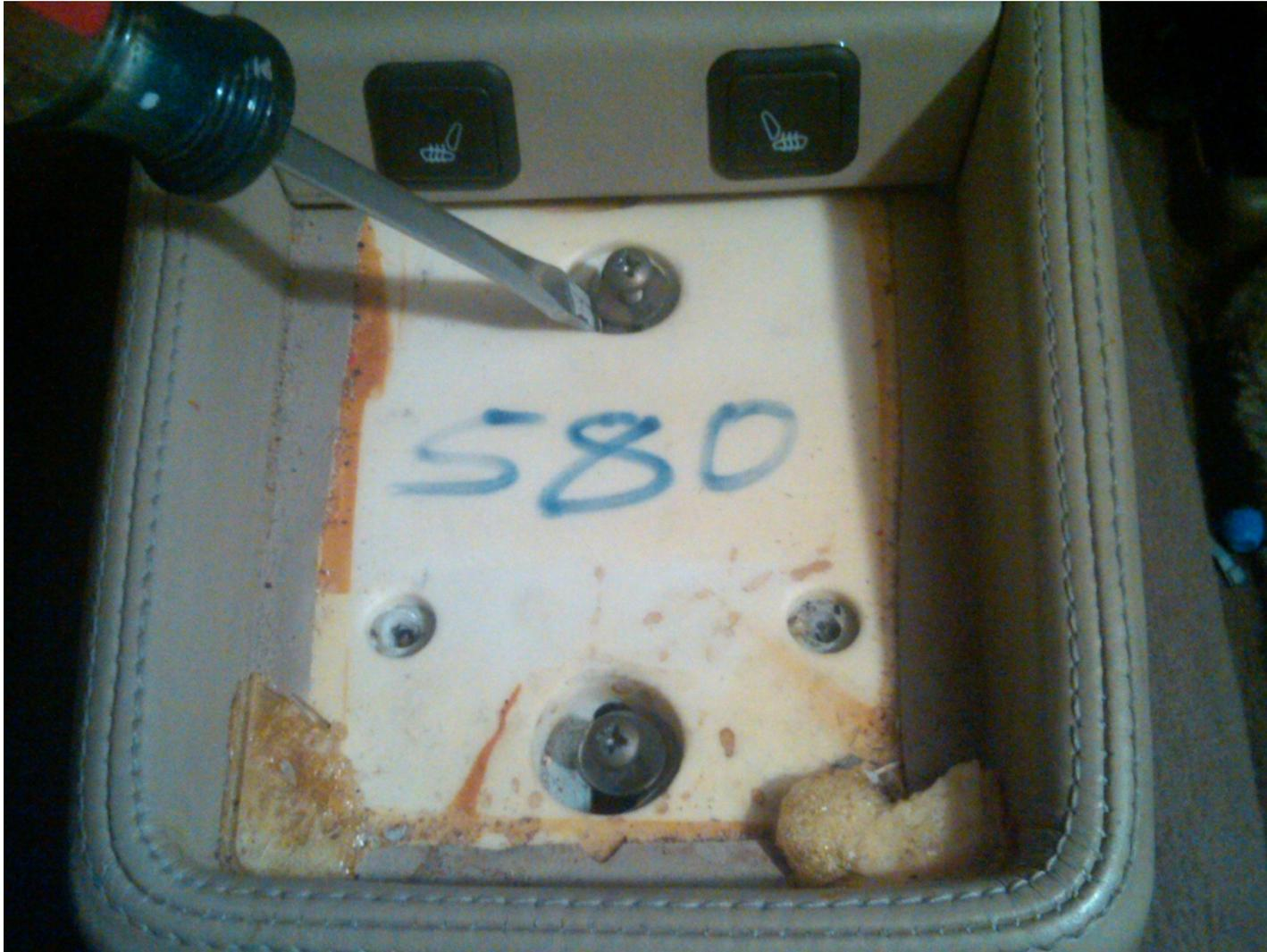
STEP-4 Push the retaining clip in an push the entire unit out the front
