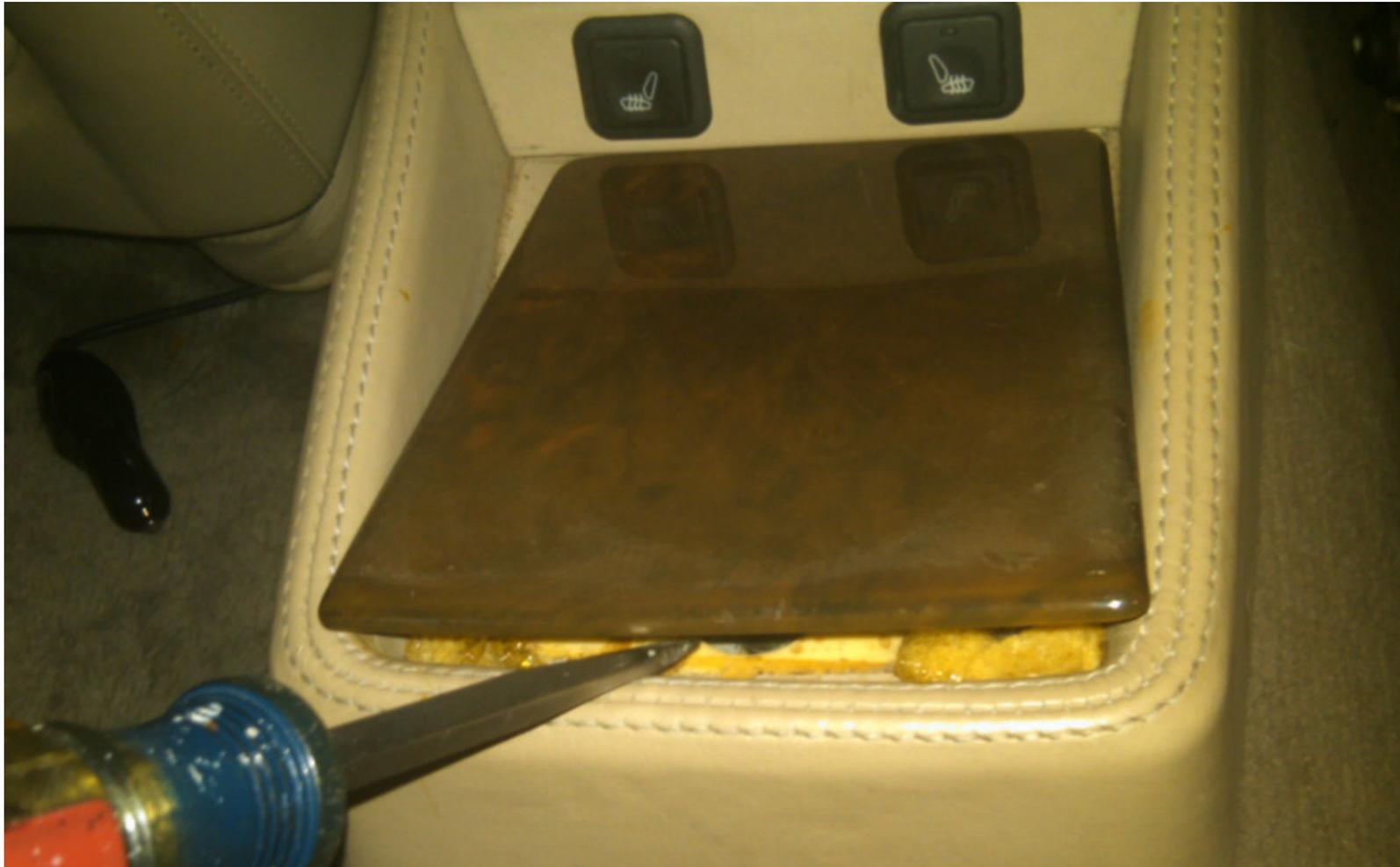
STEP-3 Remove the 2 phillips screws and remove the console
