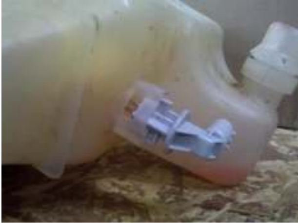
Figure 4 Level Sensor Fitting after it is rotated to allow removal
