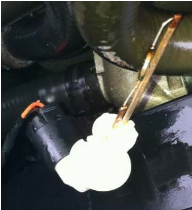
Figure 5 Level sensor after removal from tank
