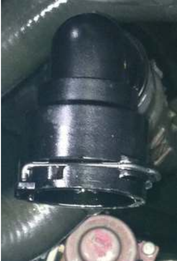
Figure 6 Primary Overflow fitting, showing wire C Clip in Locked Position
