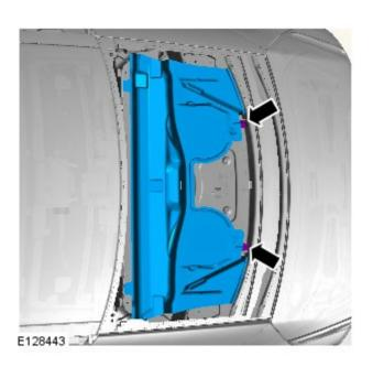
1. CAUTION: Make sure that the noise vibration harshness (NVH) material is correctly located.
