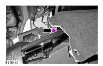
5. NOTE: Loosen the bolt, but do not fully remove.
