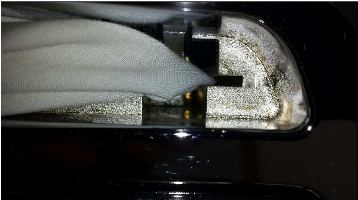
Here is the button with the flat spring and the 2 rubber stoppers. The 2 areas highlighted need to be cleaned of grease.
