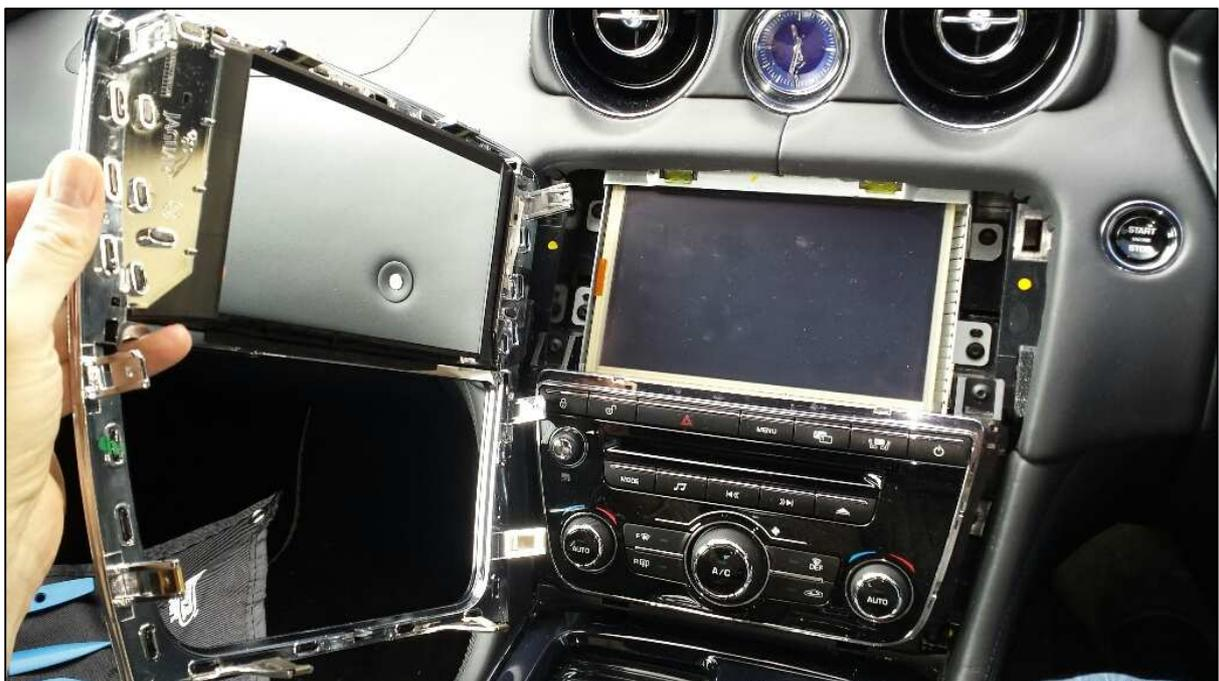
You then need to unscrew the trim below the screen. There are 4 screws to loosen at each corner.
