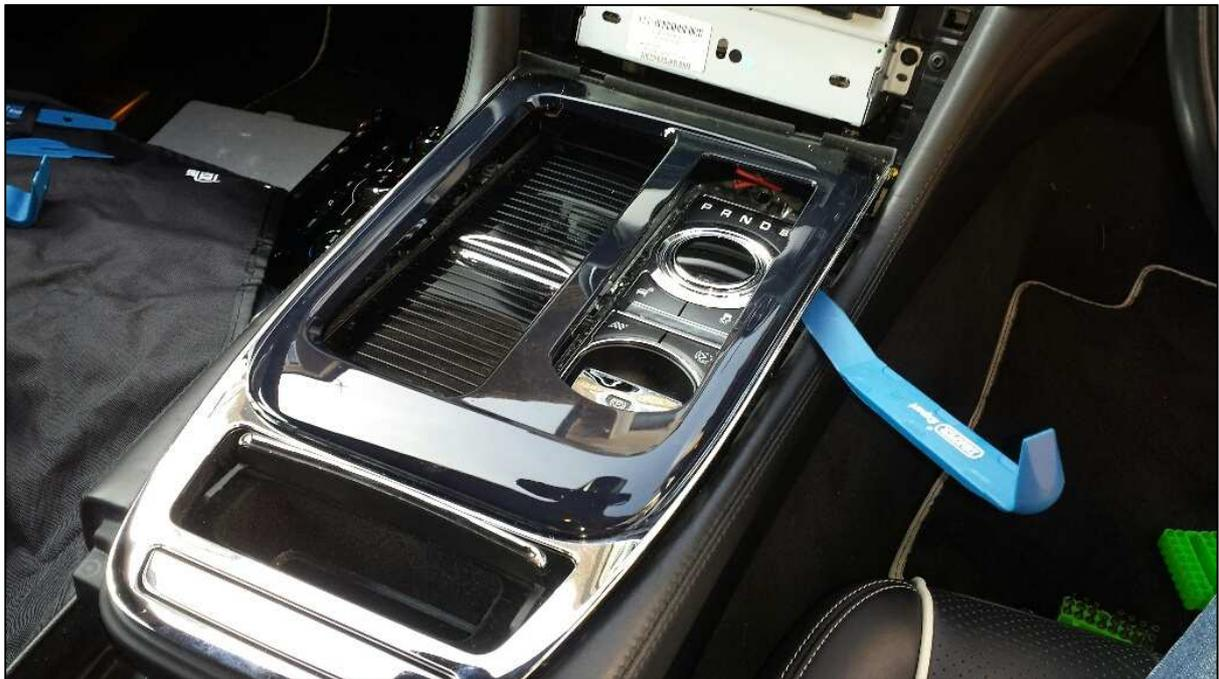
You can then lift out the trim and unplug the electric cables at the back to free the trim.
