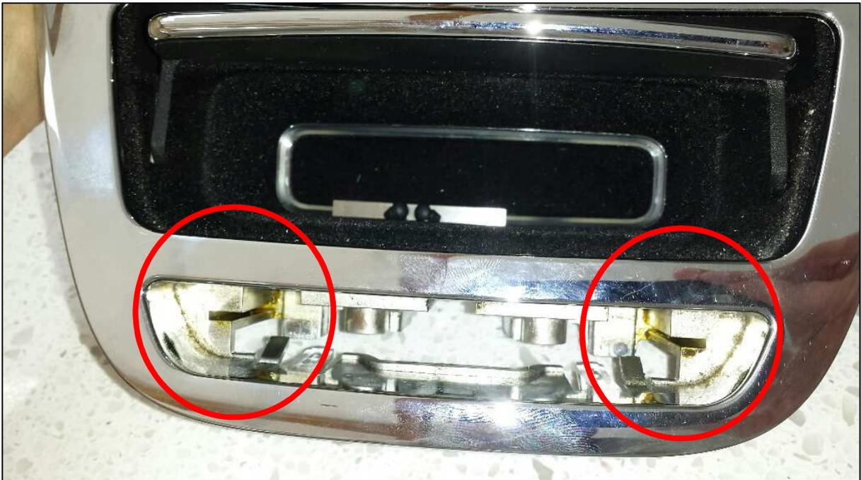
Using the white spirit and a paintbrush I cleaned out the grease. I also wrapped a cloth around a flat screwdriver to get into the groove.
