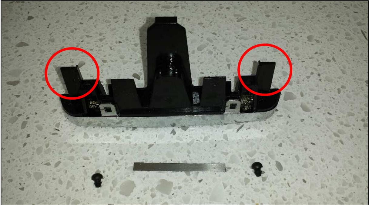
Here is a picture of the cleaned, assembled button. Take note of the 2 rubber stoppers.
