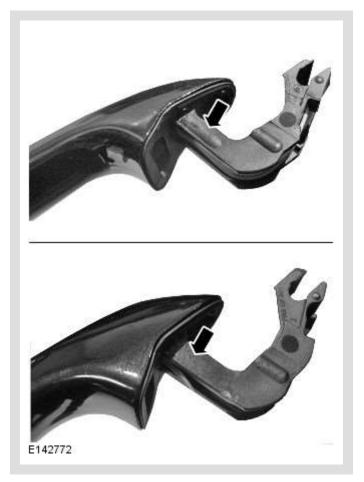
Using a suitable tool remove the moulded rib on both sides of the handle, shown in graphic E142772.
