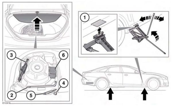
Before raising the vehicle slacken but do not remove the wheel nuts.
