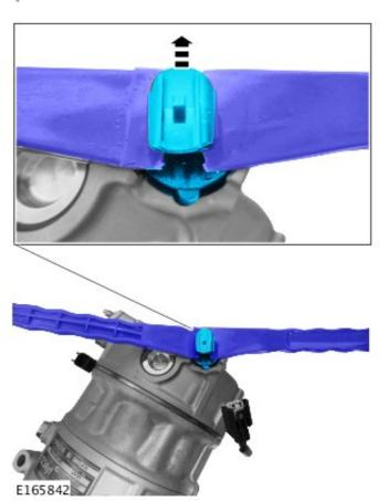
Using suitable tools, release the DPS valve.
