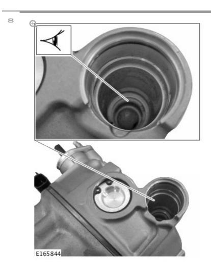
Inspect the inside wall of the A/C compressor cylinder head for scratches, scoring, or foreign material.
