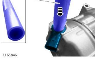
Install the DPS valve, apply a downward pressure by hand. Using a suitable tool if required, press fully into position to allow installation of
