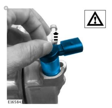
Remove by hand the DPS valve from the A/C compressor cylinder head, and discard.
