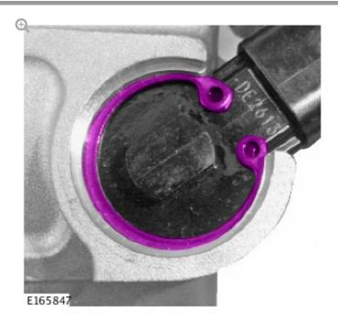
Using a suitable tool, install the new circlip supplied in the kit.
