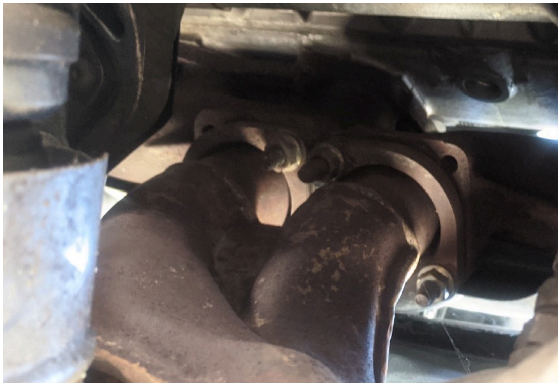
Your studs will look like this unless recently replaced.
