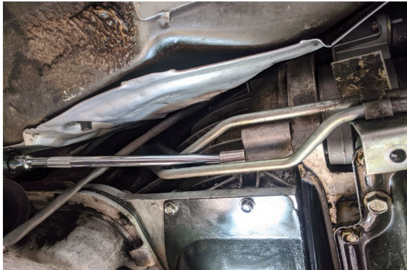
Wobble extension on lower starter motor bolt
