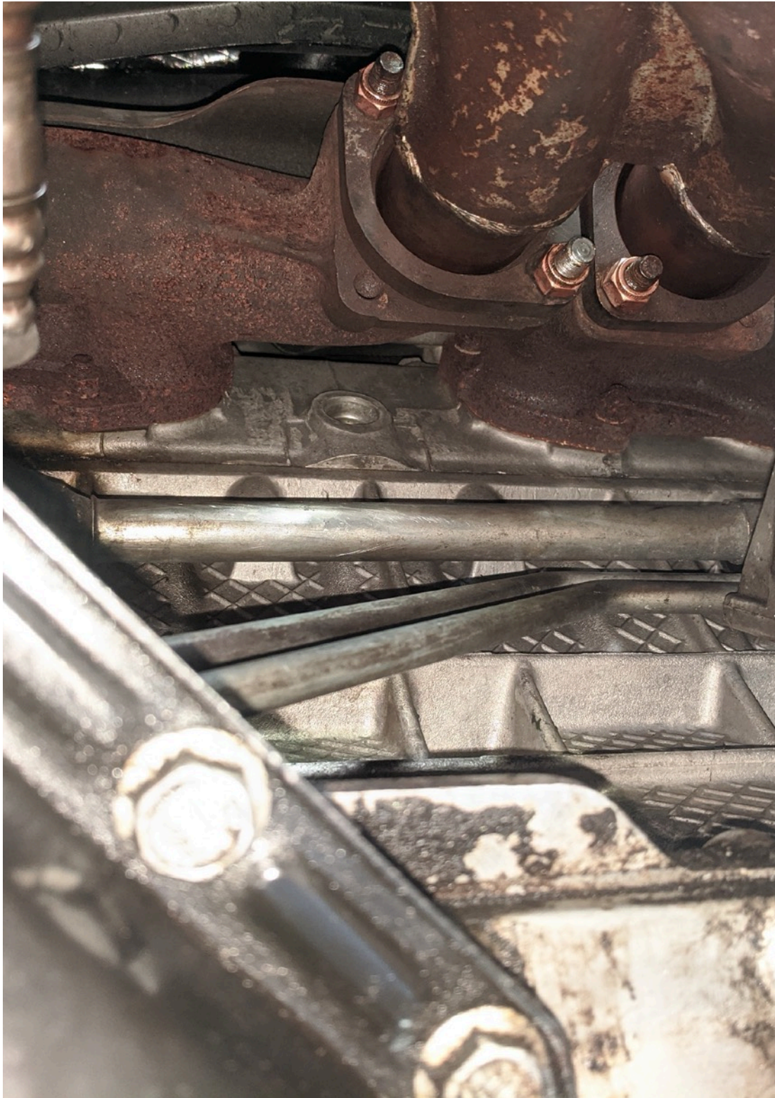
Location (Three new exhaust nuts and one new stud)
