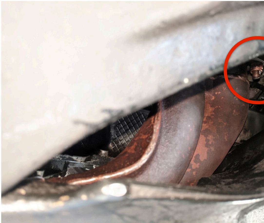
Fourth front stud visible from wheel arch
