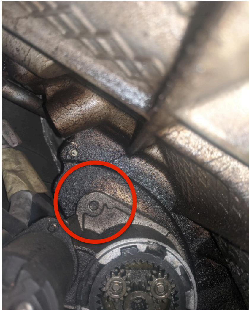
Upper bolt thread end visible for lubrication
