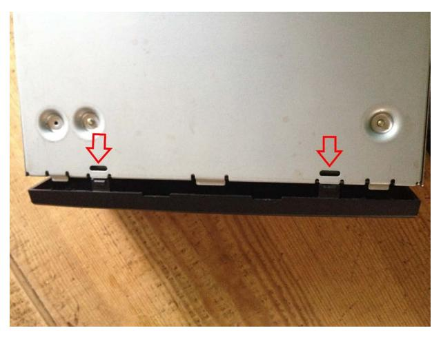
**4.**With fascia removed undo four screws, one on the front and three on the back of the drive and remove top cover.
