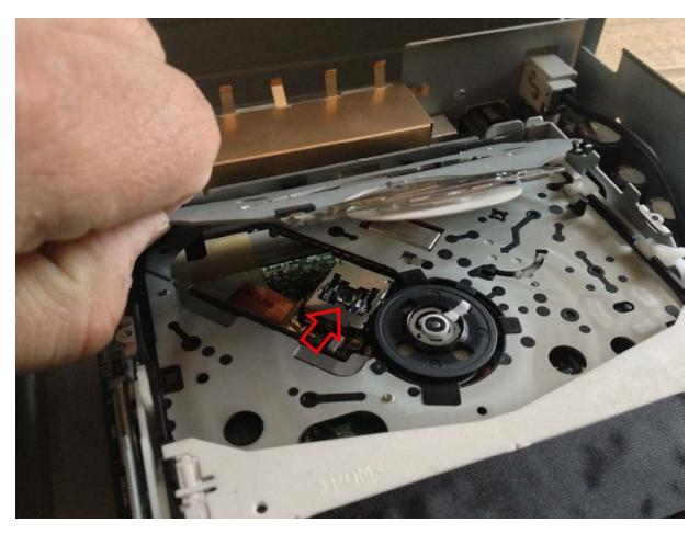
Now the fun part, adjusting the power of the laser (by doing that you can force the old laser to give bit more effort while reading the disc, **BUT AT THE SAME TIME YOU WILL GO OVER THE THRESHOLD SET BY MANUFACTURER AND CUT SHORT LASERS LIFESPAN**)
