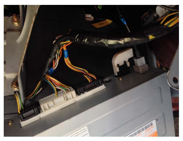
**3.**Looking at the bottom of the drive press two latches in while pulling the fascia, then swivel it to remove it completely from top latches.
