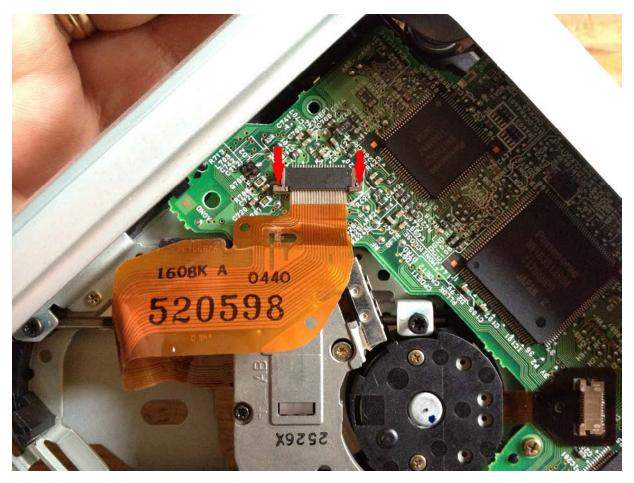
**10.**And here it is, on the photo below you can see the potentiometer which you have to turn **ANTICLOCKWISE** to let some more juice to the laser, turn in quarters or if your laser is refusing to read even genuine DVD try half turn at the time then stick it back in the car check if your disc is working, if not turn the potentiometer bit more etc.
