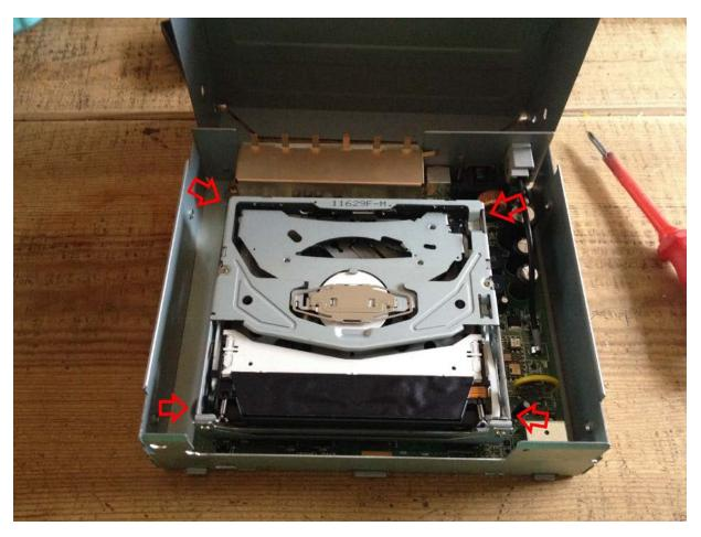
**8.**Lift the assembly taking care not to damage the ribbon, lift the brown latch up with your nail (or if you've just cut your nails use flathead screwdriver/ask missus for help) the ribbon will just pop out and you will be able to remove the assembly.
