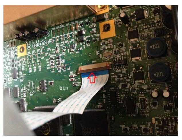
**9.**This step is actually optional but to get better access, you can remove the laser assembly's ribbon, by sliding little brown latches as indicated on the photo.
