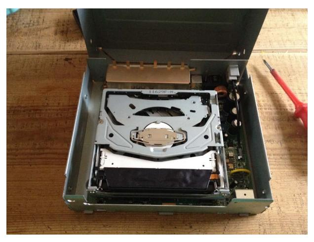
**5.**If you planning on cleaning the lens, remove two small screws and remove the frame that holds the top drive mechanism.
