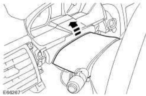
3 . Remove the steering column multifunction switch.
