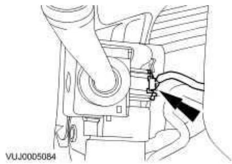
5 . Remove the steering column multifunction switch RH switch.
