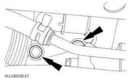
17 . Disconnect the secondary air injection (AIR) control valve to exhaust manifold tube.
