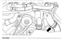
8 . Disconnect the engine coolant temperature (ECT) sensor electrical connector.
