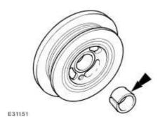
CAUTION: The screw thread in the crankshaft must be cleaned out before a new crankshaft pulley bolt is installed.
