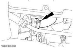
16 . Remove the power steering pump lower retaining bolts.
