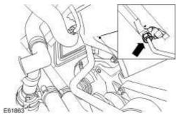
27 . Remove the AIR control valve to exhaust manifold tube.
