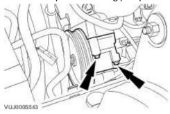
21 . Remove the accessory drive belt idler pulley.
