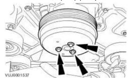
9 . Remove the accessory drive belt idler pulley.
