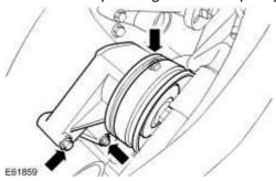
23 . Remove the supercharger belt tensioner.
