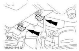
9 . Install the power steering pump mounting bracket.
