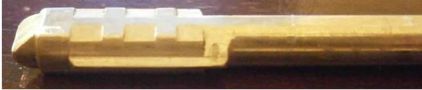
Going from the base of key to tip of key the T code for this key is T421212.
