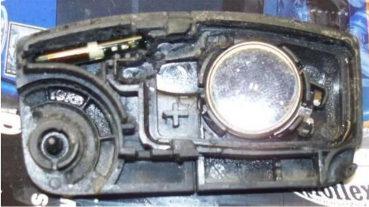
Transponder chip: antenna is the copper looking side
