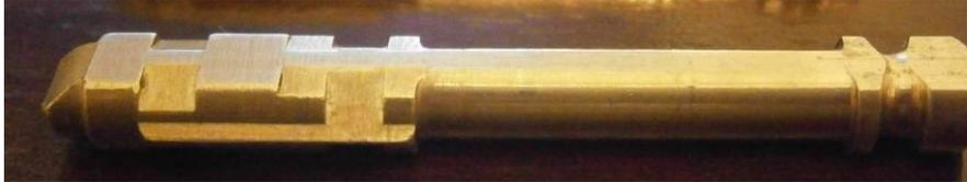
Going from the base of key to tip of key the T code for this key is T242113.
