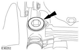
16. NOTE: Place a suitable cloth around supercharger fill port.
