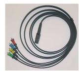
The Secondary Ignition Transducer Cables are used to connect the VMM to either Secondary Ignition Transducer Clips or COP Clips to perform ignition routines. These cables can be used on a breakout box with Probe Tip Adapter Kit #2.
