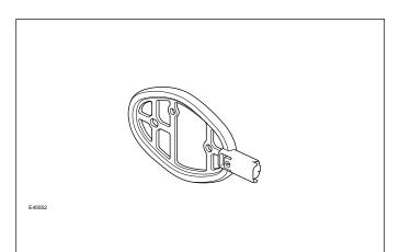
The initiators are located at the front of the front wheel arches and at the rear of the rear wheel arches. The TPMS system has four initiators. Each initiator has a connector which connects with the body harness.
