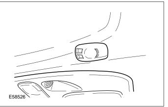
The microphone is located above the driver and is attached to the headliner.
