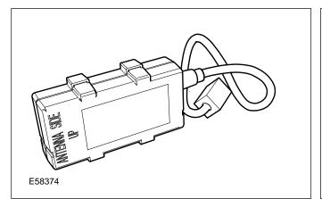
The Bluetooth upgrade module has one electrical connector and communicates with the PSE module by it's own proprietary communications bus.
