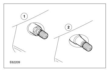
Wheels fitted with TPMS can be visually identified by the external metal lock nut and valve (1). All Jaguar non-TPMS wheels have a rubber valve fitted (2).
