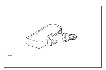
The TPMS system uses 'active' tire low pressure sensors which are mounted on each wheel, inside the tire cavity. The sensor is retained in position by the valve attachment to the wheel structure. The sensors transmit RF signals at either 315 MHz or 433 MHz dependent on market requirements.
