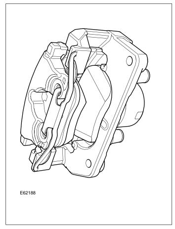
With the increased caliper piston size, the brake discs have also been enlarged from 300 mm to 326 mm.
