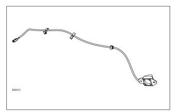
The TPMS external antenna is located at the rear of the vehicle and is mounted between the spare wheel well and rear subframe.
