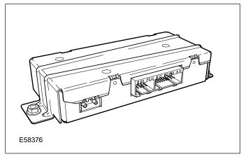
The voice activated control module is fixed to a bracket which also supports the PSE and the navigation control module. The voice activated control module stores up to 40 voice tags.
