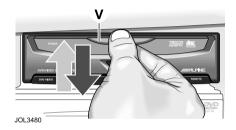
**Note:** The ignition switch must be in position **I** or **II** to insert or eject a DVD.
