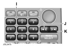
Press and release button (K) to seek up, or button (J) to seek down, to the next station.
