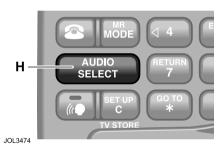
Press button (**H**) repeatedly until the name of the audio source that you wish to listen to is shown on the switchpack display.
