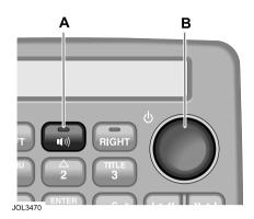
Press the rotary control (**B**) to switch on.
