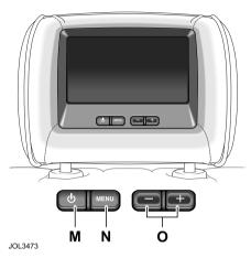
Press button (**M**) to switch on the video display screen.
