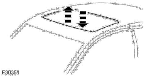
3. Adjust the front edge of the roof opening panel glass to between flush and 1 mm (0.04 in) low.
