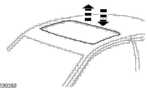
4. Adjust the rear glass edge to between flush and 1 mm (0.04 in) low.
