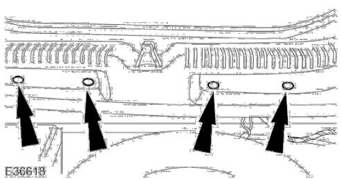
2. Remove the luggage compartment trim panel lower retaining clips.
