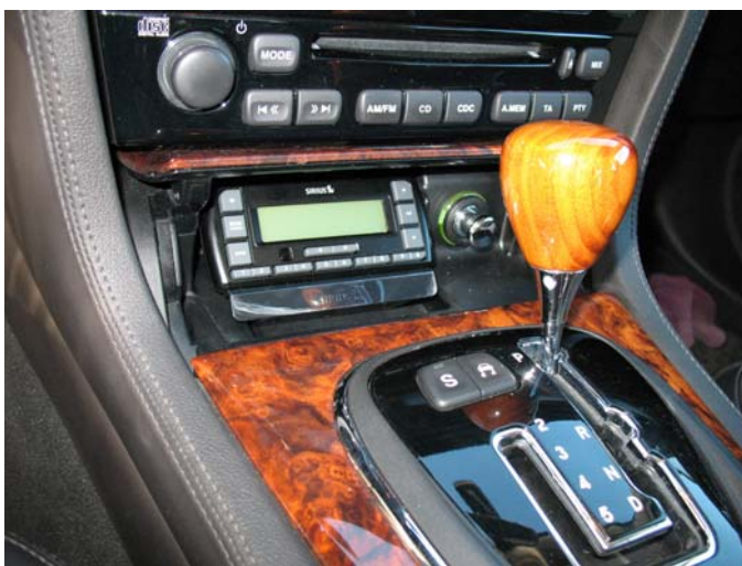
Satellite radio installed with fabbed back plate spacer and Velcro. You have to mess with the angle to allow the ashtray cover to still close
