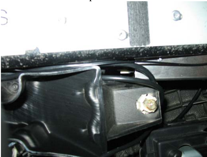
The ACM unit itself goes up behind the glovebox. Hopefully I found a flat enough area for the double sided tape to stick to!
