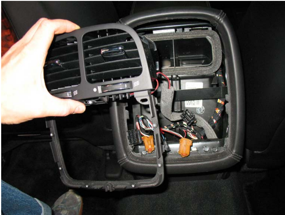
Rear vents pull off but still have some connectors to remove
