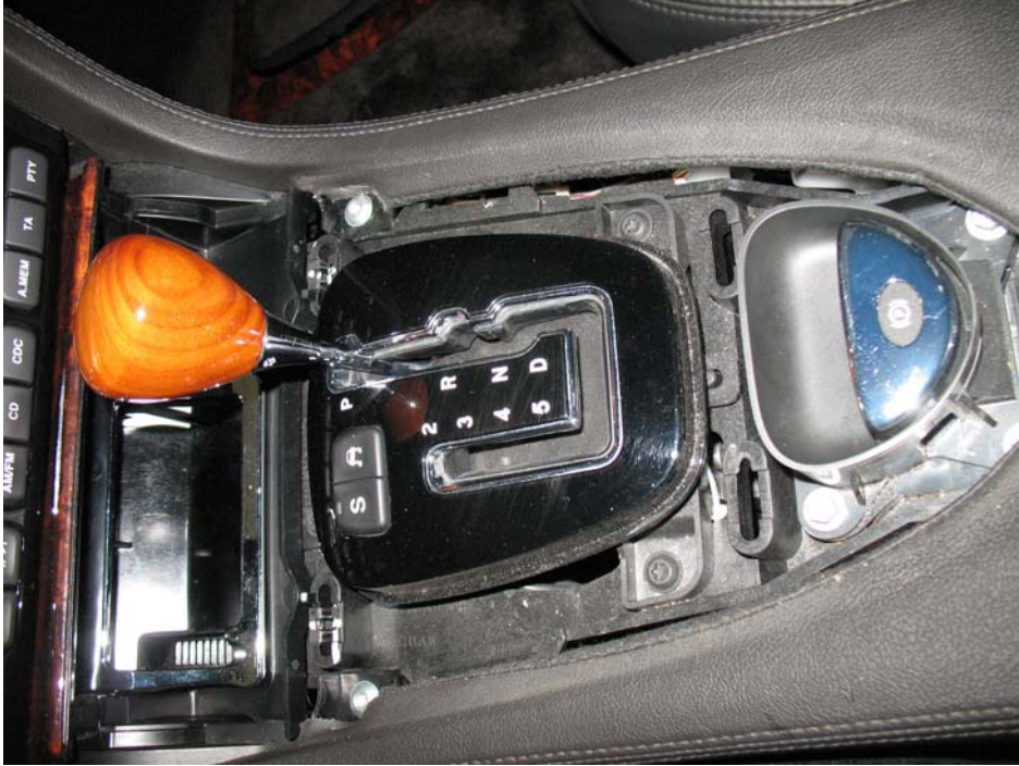
Trim around gear shifter is a friction fit and can be carefully prised off
