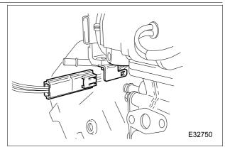
9 Remove the throttle body to induction elbow securing bolts.
