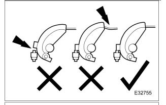
WARNING: For vehicles with the plastic adjustment nut; after correct cable adjustment, you must install a ratchet tie strap to fully retain the adjuster nut in its location within the abutment bracket. Please refer to recall action r466.
