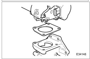
11 Remove the throttle cable and intake duct bracket.
