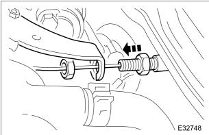
CAUTION: Under no circumstances should the quadrant be held clear of the throttle stop by cable tension. Ensure there is no tension or slack in the cable.
