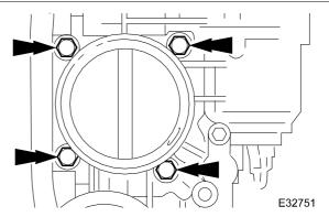
10 Remove the throttle body from the induction elbow, discard the gasket, and blank off the inlet tract to prevent ingress of foreign matter.
