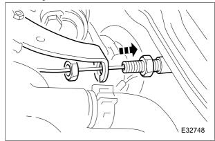
Remove the coolant hoses and install suitable blanking plugs.
