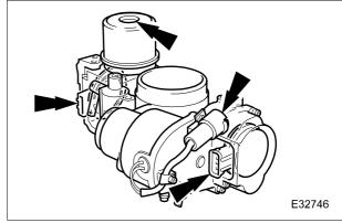
4 Rotate the throttle quadrant to allow disconnection of the inner cable.
