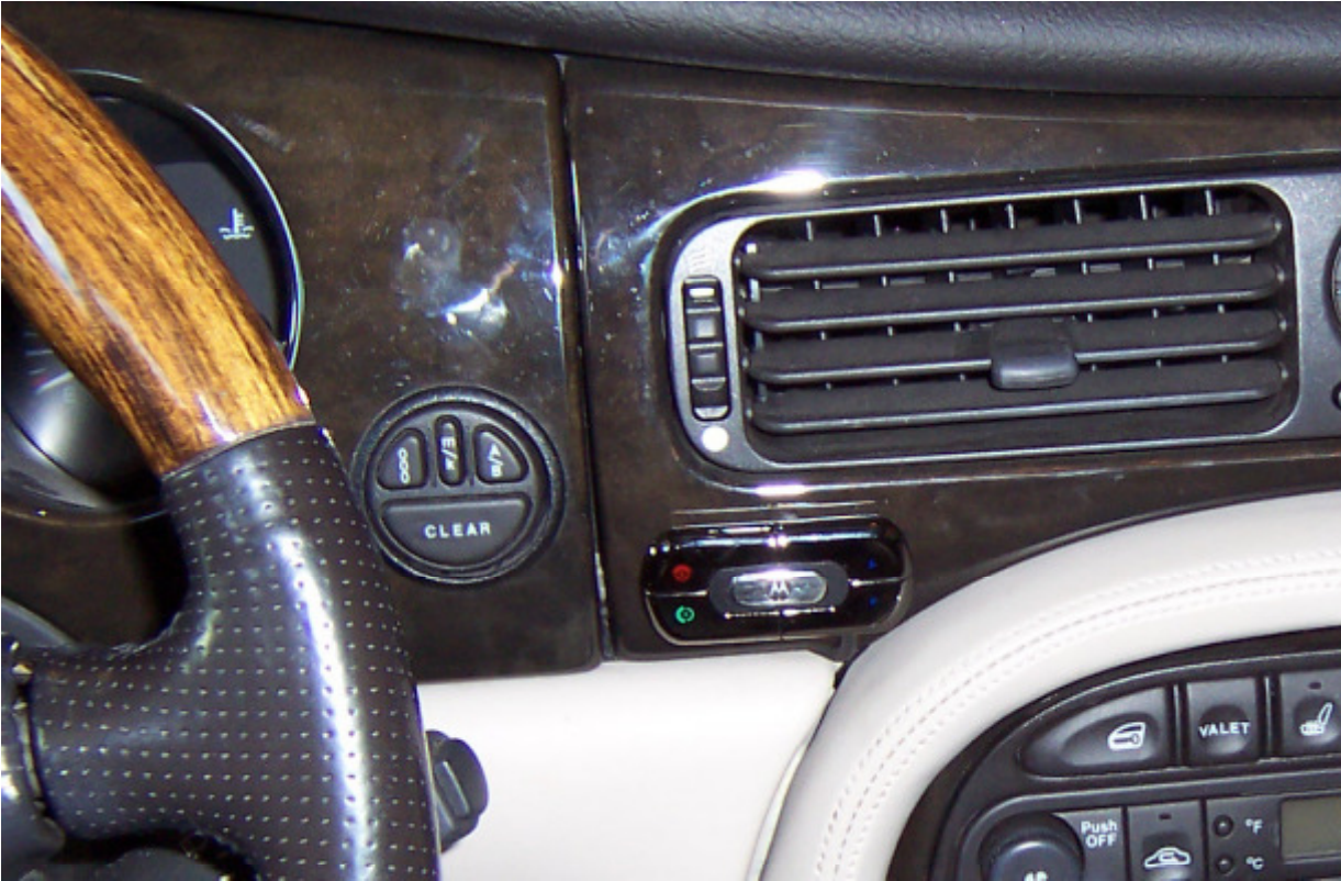
I routed the wires behind this trip panel toward the drivers side of the car, then behind the instrument panel trim. From there I routed it to the center console to the car kit module. There is plenty of room to pull the 8-pin connector through. You must however, remove
