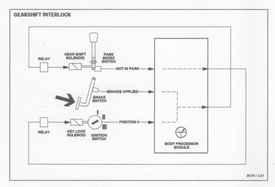
A gearshift interlock override is provided in the gear selector "J" gate. Remove the plastic screw at the left front side of the selector lever to access the release.
