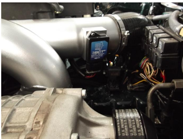
100mm main air inlet pipe with new air flow meter
