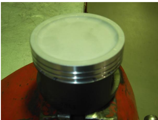
Forged piston, Ceramic and Teflon coated. Bottom end ready
