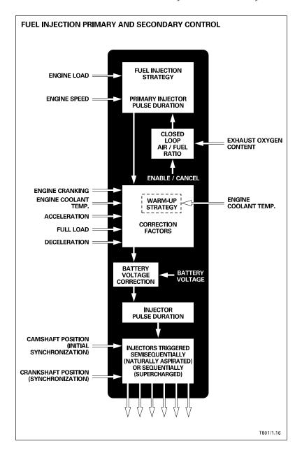
Sequential fuel injector pulsing is ECM controlled. The ECM "learns" the compression stroke synchronization at each engine start from the camshaft position sensor (CMPS) and crankshaft position sensor (CKPS) inputs. After the firing synchronization is learned, the ECM uses the CKPS input for engine speed and position. Refer to the CMPS description on page 27 and the CKPS description on page 26.
