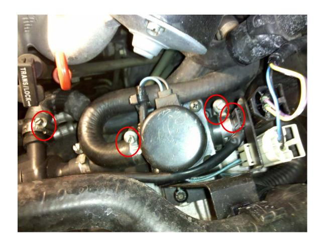
Since I had replaced the Pump-to-valve hose last summer when I replaced the radiator and bypass hoses, and flushed & renewed the coolant, I was keen to leave that in place as an asy and just disconnect the affected hoses. After loosening the affected hose clamps, I determined that to be an unworkable plan
