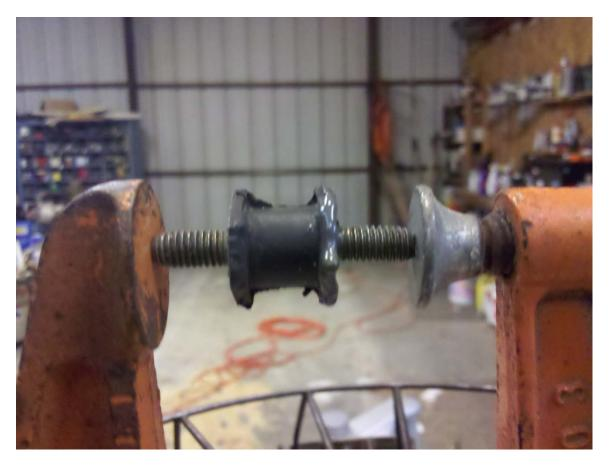
I mixed up a bit of 2-part epoxy, carefully clamped both pieces together, then suspended it over the kerosene heater I was using to make the shop habitable for middle-aged man work. Eventually, I had gone as far as I could without remounting the WV, so I took the heat gun to it all 'round and cured it up quickly
