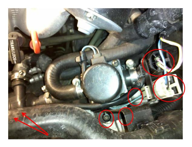
So I disconnected the electrical connectors and removed 3 fixing nuts from the valve bracket and two from the pump mounting (not shown) and removed it as an asy, connected by the hose.
