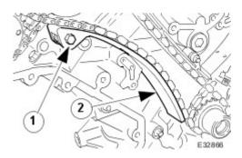
23 . Remove the chain from the VVT unit and from the crankshaft pulley.
