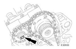
19 . Loosen the bolt which secures the VVT unit to the camshaft.
