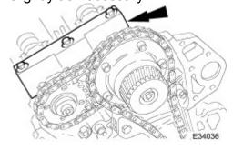
18. Loosen the bolt which secures the sprocket to the camshaft.
