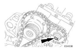
26 . Loosen the bolt which secures the VVT unit to the camshaft.
