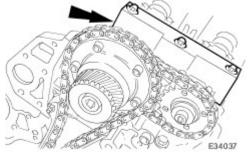
25 . Loosen the bolt which secures the sprocket to the camshaft.
