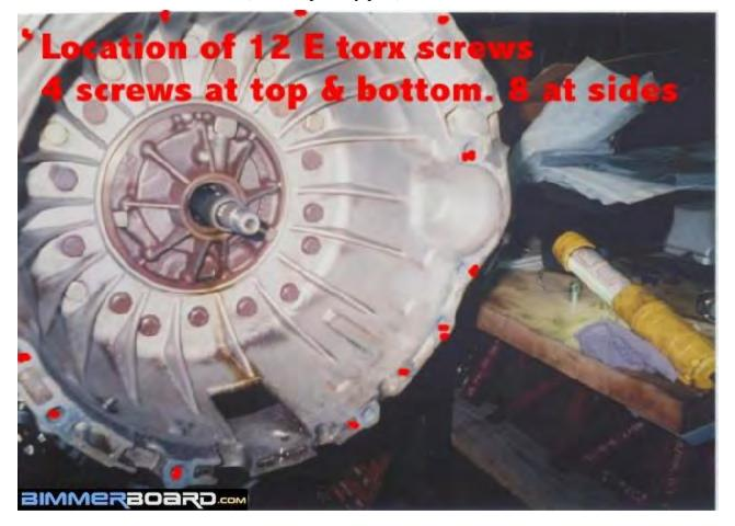
25) Wipe seal area clean and using a pick or similar tool remove front pump shaft seal snap ring.
