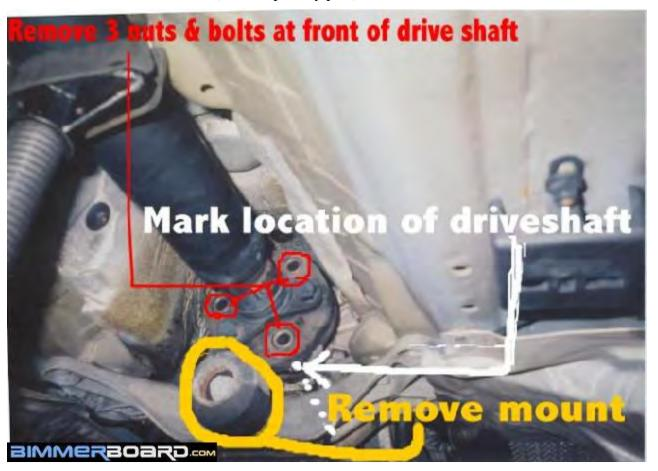
13) Mark rear drive shaft location and remove 8 nuts that secure drive shaft to differential.
