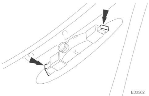
7. Release retaining clips and remove sidemarker lamps/reflectors from bumper.
