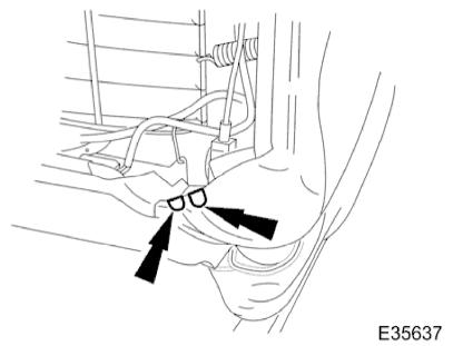
2. Release back finisher from the side securing clips.
