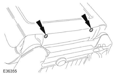
1. Slacken and remove the two back finisher lower securing screws.
