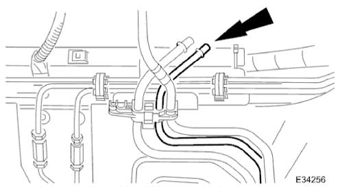
7. At the engine bay bulkhead, locate the quick fit connector between the underfloor fuel feed pipe and the fuel pulse damper.
