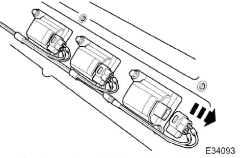
4. Detach harness from retaining clips as necessary and disconnect relevant coil connector.
