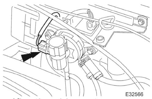
3. Disconnect the purge valve harness connector.
