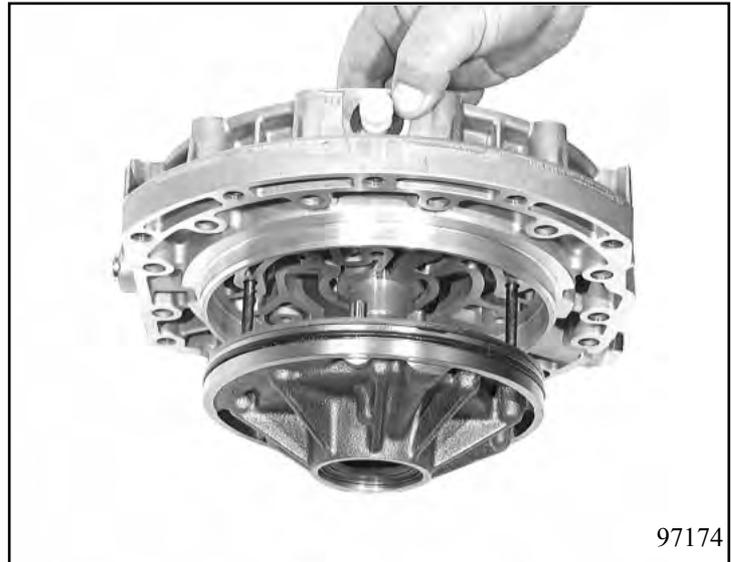
Attach shim 02.260 to the stator shaft using petroleum jelly.
