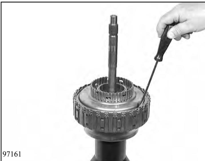
Put inner disc carrier C 72.190 into cylinder B and secure it with snap ring 72.200.
