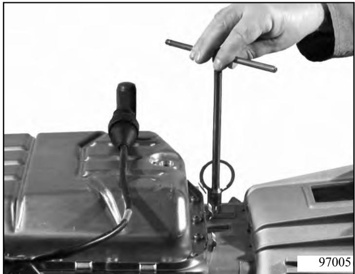
Remove the protective transport cap from the selector shaft.
