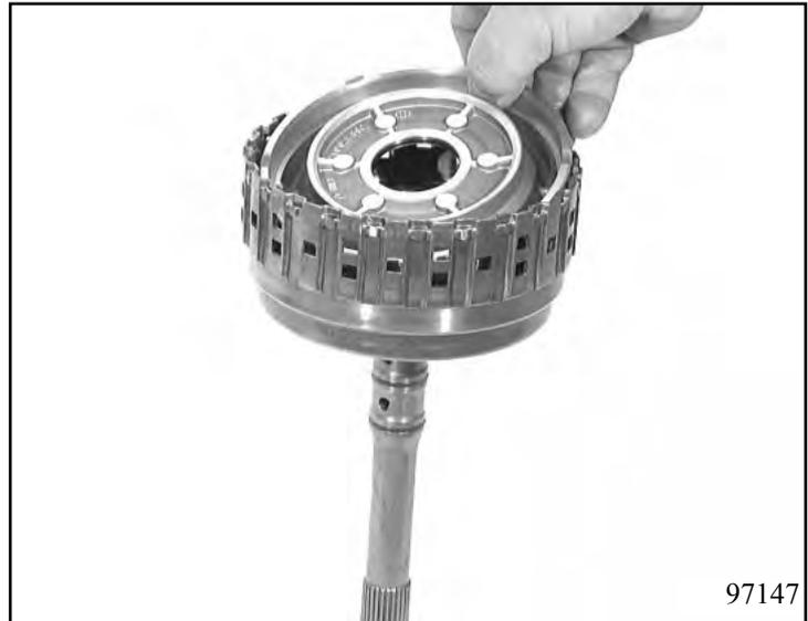
Put a new O-ring 70.070 onto oil dam 70.060. Insert cup spring 70.050 into cylinder A and press in the oil dam. Using assembly bracket 5x46 001 499, press down the oil dam in the mandrel press, and secure it with snap ring 70.080.
